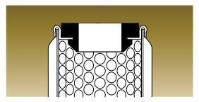
Rosedale seals are specially shaped to hold in place mechanically, like a grommet. There's little chance they will be dislodged and lost in handling. They are made in different thicknesses to provide seven different standard overall element lengths.
